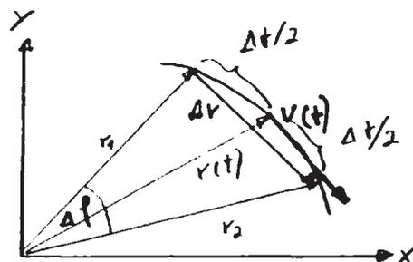
$$\begin{matrix} X_{31} = X_{30} - X_{10} \\ Y_{31} = Y_{30} - Y_{10} \end{matrix} \quad X_{31}, Y_{31} \xrightarrow{RP} \varphi_v, |\vec{r}_{13}| \quad \boxed{|\vec{v}| = \frac{|\vec{r}_{13}|}{\Delta t_v}}$$
