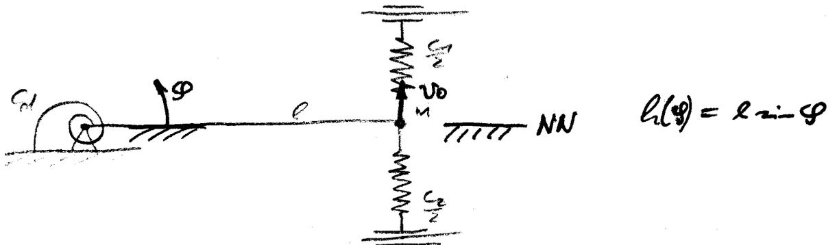
$$1) V(\varphi) = mgl \sin \varphi + \frac{1}{2} \left( \frac{c_1}{2} + \frac{c_2}{2} \right) l^2 \sin^2 \varphi + \frac{1}{2} c_d \varphi^2$$
